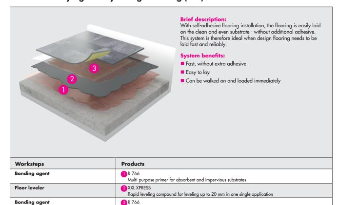
**Multi-purpose primer for absorbent and impervious substrates** (Also as a bonding agent before direct bonding of floorings)
