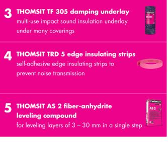
Vinyl design coverings (LVT) THOMSIT K 190 F – fiber-reinforced PVC and rubber adhesive THOMSIT AS 2 – fiber-anhydrite leveling compound THOMSIT TRD 5 – self-adhesive edge insulating strips THOMSIT TF 305 – THOMSIT-Floor<sup>®</sup> damping underlay Prepared substrate
